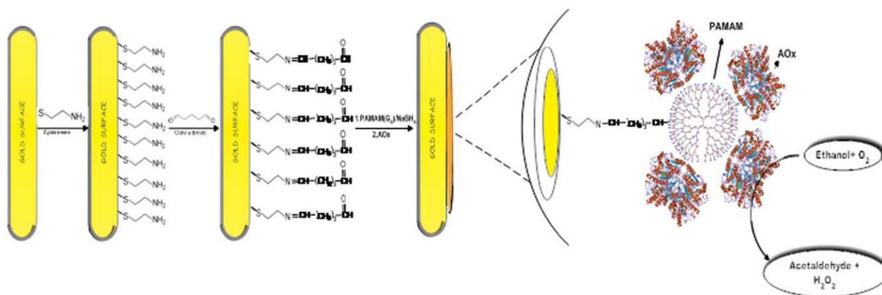
Scheme 1. Surface modification and immobilization procedure.
