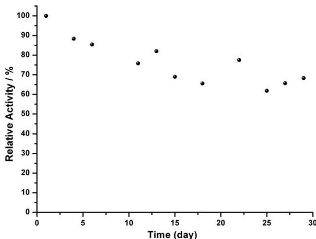
Figure 9. Storage stability of PAMAM/AOX biosensor (in sodium phosphate buffer, 50 mM, pH 7.0; 25°C; -0.7 V).
