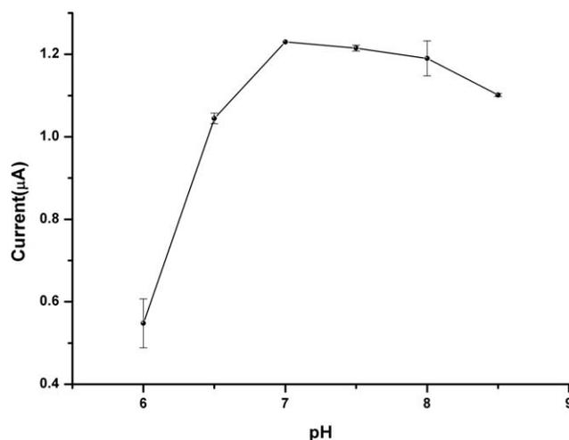
Figure 1. Effect of pH (sodium citrate buffer at pH 6.0; 6.5, sodium phosphate buffer at pH 7.0; 7.5; 8.0 and Tris-HCl buffer at pH 8.5, 25°C,  $-0.7$  V,  $[EtOH]$ ; 0.5 mM).
