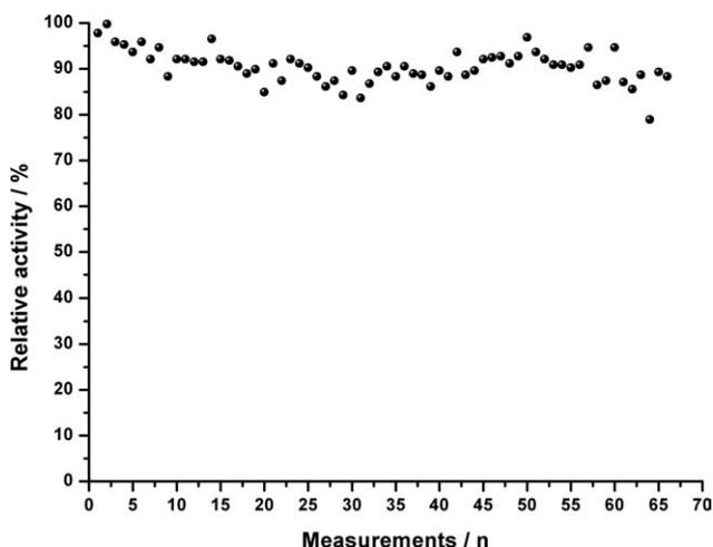
Figure 8. Relative activity (%) vs. consecutively injections of 0.7 mM ethanol in 50 mM sodium phosphate buffer, pH 7.0 during 210 min.
