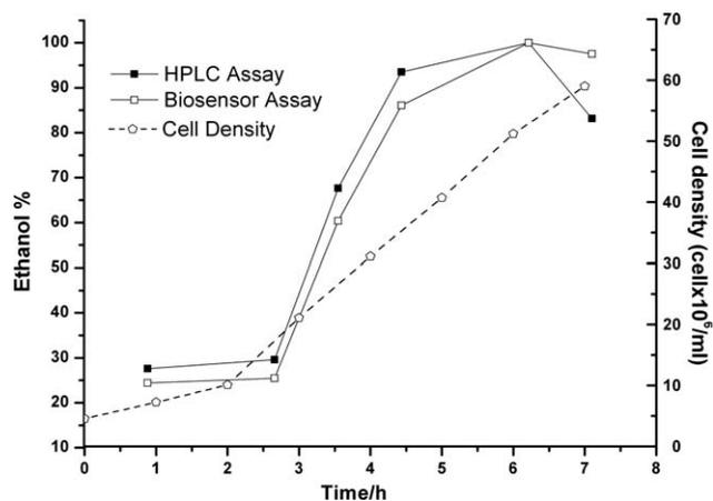
**Figure 10.** Time depending alcohol concentration in fermentation medium (in sodium phosphate buffer, 50 mM, pH 7.0; 25°C;  $-0.7$  V).
