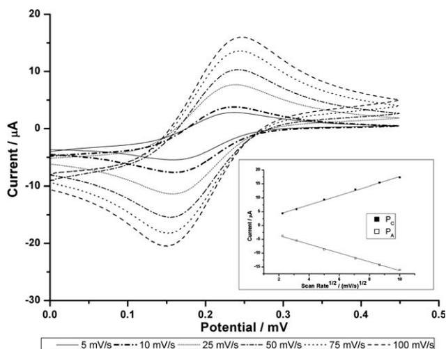
Figure 4. Cyclic voltammograms of cysteamine/PAMAM modified electrode in 50 mM pH 7.0 sodium phosphate buffer with the presence of 5 mM  $[\text{Fe}(\text{CN})_6]^{4-/3-}$  at 5, 10, 25, 50, 75, 100 mV/s. Inset: Plots of anodic and cathodic peak currents vs. scanrate<sup>1/2</sup>
