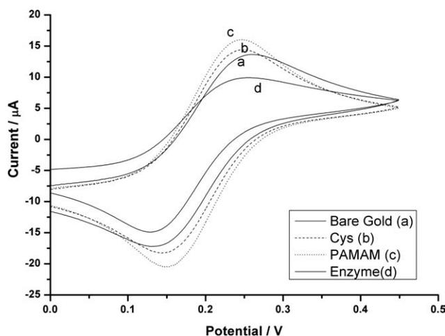
Figure 3. Cyclic voltammograms of bare gold electrode (a), cysteamine (b), cysteamine/PAMAM (c) and cysteamine/PAMAM/AOX (d) in 50 mM sodium phosphate buffer, pH:7.0 with the presence of 5 mM  $[\text{Fe}(\text{CN})_6]^{4-/3-}$  at 100 mV/s
