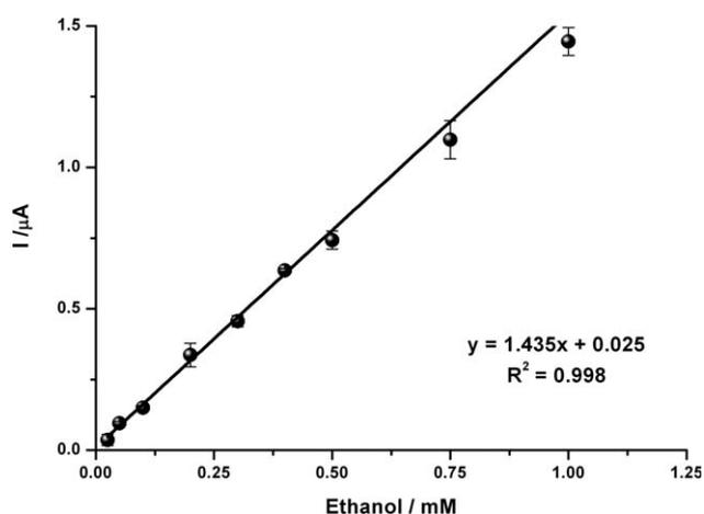
Figure 5. Calibration curve for ethanol (in 50 mM sodium phosphate buffer, pH 7.0; 25°C; -0.7 V).
