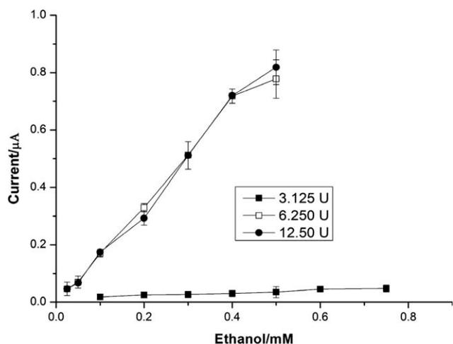
Figure 2. Effect of enzyme amount on the biosensor response (in sodium phosphate buffer, 50 mM, pH 7.0; 25°C, -0.7 V).
