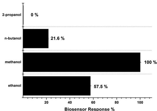
Figure 7. Comparison of the biosensor response for the different aliphatic alcohols (in phosphate buffer 50 mM, pH 7.0; 25°C; -0.7 V, [Alcohol]: 0.5 mM).
