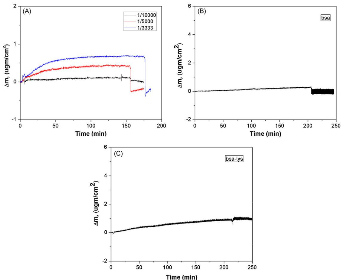
**Fig. 4.** Specificity of lysozyme imprinted QCM nanosensor. (A) real-time lysozyme detection from natural source in different dilutions; (B) real-time albumin response from single component aqueous solution; (C) real-time QCM response from aqueous solution containing albumin/lysozyme mixture.
