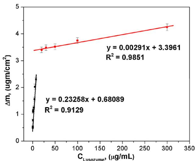
Fig. 3. Concentration dependency of lysozyme imprinted QCM nanosensor.
