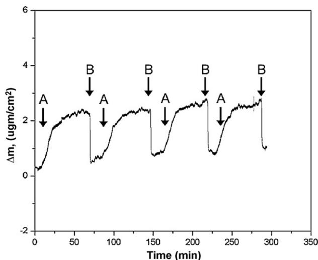
**Fig. 5.** Reproducibility of lysozyme imprinted QCM nanosensor response. (A) Adsorption; (B) Desorption.
