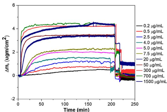
Fig. 2. Real-time lysozyme detection with lysozyme imprinted QCM nanosensor.
