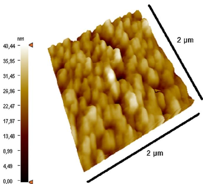
Fig. 1. Atomic force microscopy picture of lysozyme imprinted QCM sensor.
