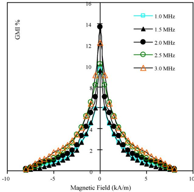
Fig. 3. The magnetic field dependence of the GMI ratio for the diamagnetic organic thin film coated samples.
