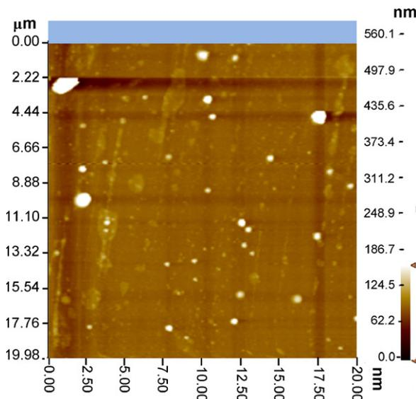
Fig. 4. 2D topography image of uncoated Co-based amorphous ribbon. The image size is 20  $\mu\text{m} \times 20 \mu\text{m}$ .
