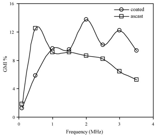
Fig. 1. The frequency dependence of the GMI ratio for the Co-based amorphous ribbons.
