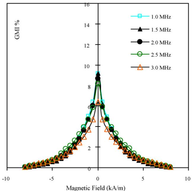
Fig. 2. The magnetic field dependence of the GMI ratio for the uncoated samples.
