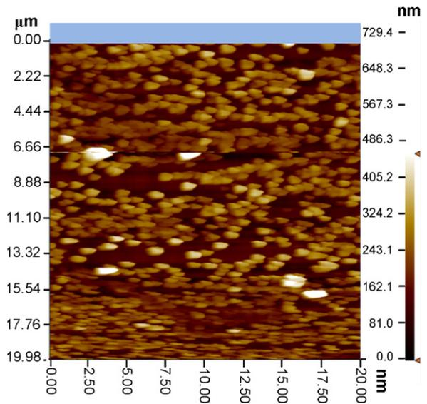
Fig. 5. 2D topography image of organic coated Co-based amorphous ribbon. The image size is 20  $\mu\text{m} \times 20 \mu\text{m}$ .
