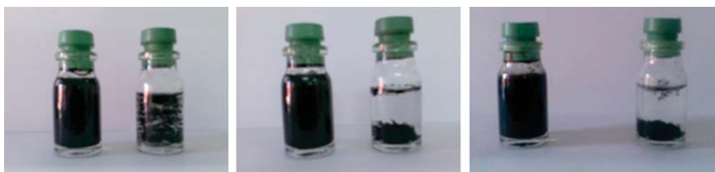
Fig. 10. The appearance of the dispersions of PEGylated MWCNTs and MWCNTs in water after 0, 15 minutes and 54 days of preparation.
