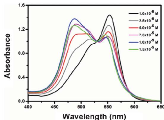
**Fig. 4** The absorption spectra of PyY in the GO aqueous dispersion at various dye concentrations. (The GO aqueous dispersion includes  $17 \text{ mg L}^{-1}$  GO. The spectra were normalized at the isosbestic point in order to show clearly the change of relative absorbance due to monomers and aggregates.)
