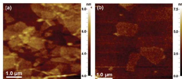
Fig. 2 Tapping mode AFM images ( $5 \mu\text{m} \times 5 \mu\text{m}$ ) of GO (a) and PyY adsorbed GO (b) on a freshly prepared mica surface.
