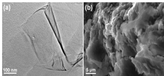
Fig. 1 TEM (a) and SEM (b) images of a GO sheet.
