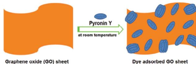
Scheme 1 Schematic illustration of a 2D GO–PyY nanocomposite in an aqueous dispersion.
