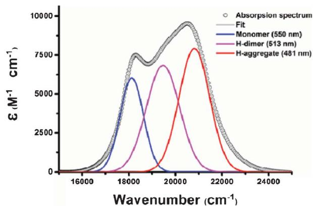
Fig. 6 Deconvolution of the aggregate absorption spectrum of  $1.0 \times 10^{-5}$  M PyY in the GO aqueous dispersion.
