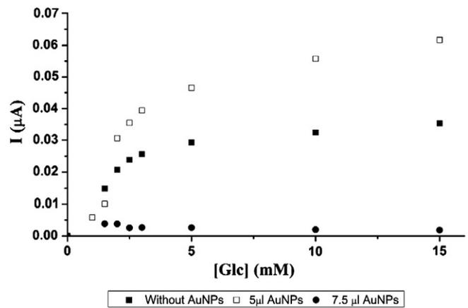
Fig. 7. Effect of the AuNPs amount on the biosensor response in 50 mM, pH 4.0 acetate buffer (1.98  $\mu\text{mol}$  FcSH; 42 U GOx; +0.35 V).
