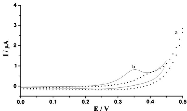
Fig. 6. Voltammograms comparing electrodes in absence (a) and presence of AuNPs (5.0  $\mu\text{L}$ ) (b) in 50 mM pH 4.0 acetate buffer (1.98  $\mu\text{mol}$  FcSH; 42 U GOx; scan rate: 50  $\text{mV s}^{-1}$ ).
