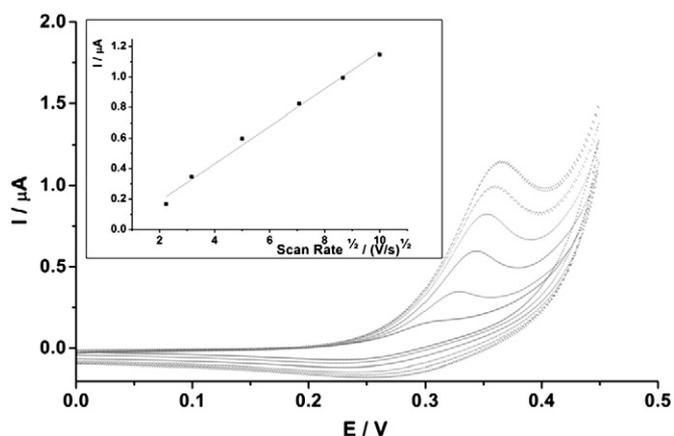
**Fig. 1.** Cyclic voltammograms of Au/(FcSH + Cyst)/PAMAM/AuNP/GOx biosensor (50 mM, pH 4.0 acetate buffer; 5.0  $\mu\text{L}$  AuNPs; 1.98  $\mu\text{mol}$  FcSH; 42 U GOx; scan rates in the range of 5.0–100  $\text{mV s}^{-1}$ ). Scan rates are 5.0, 10, 25, 50, 75, 100  $\text{mV/s}$  from inside to out.
