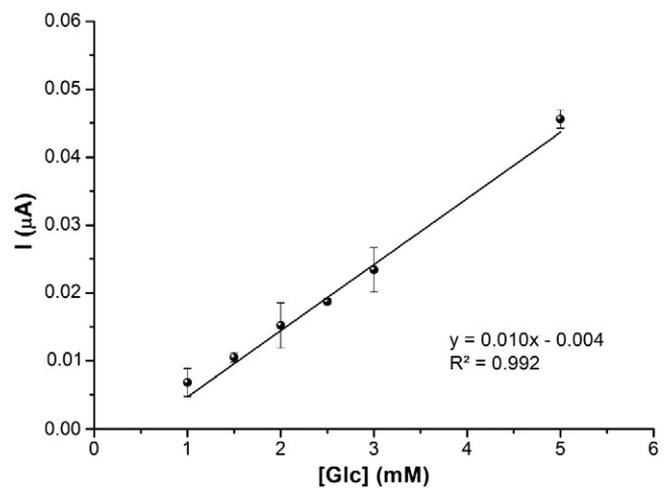
Fig. 8. Calibration plot for glucose in optimized conditions (50 mM, pH 4.0 acetate buffer; 5.0  $\mu\text{L}$  AuNPs; 1.98  $\mu\text{mol}$  FcSH; 42 U GOx; +0.35 V).
