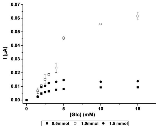
Fig. 5. Effect of the FcSH amount on the biosensor response studied by calibration plots obtained for glucose (50 mM pH: 4.0 acetate buffer; 5.0  $\mu\text{L}$  AuNPs; 42 U GOx; +0.35 V).
