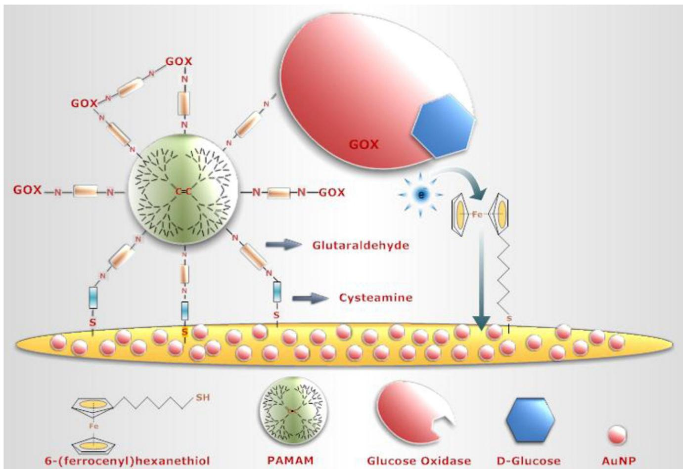
**Scheme 1.** Schematic representation of the proposed biosensor.
