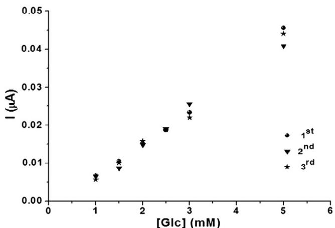
Fig. 9. Calibration plots of three different biosensor prepared on different days (50 mM pH 4.0 acetate buffer; 5.0  $\mu\text{L}$  AuNPs; 1.98  $\mu\text{mol}$  FcSH; 42 U GOx; +0.35 V).
