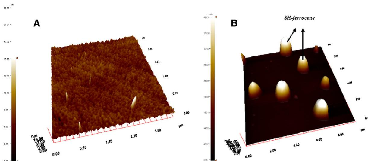
Fig. 2. AFM images of AuNP modified (A) and AuNP/SH-ferrocene modified (B) gold surface.
