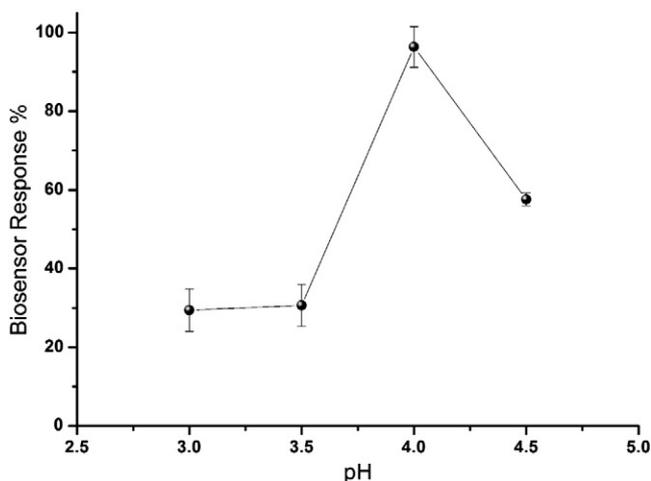
Fig. 3. Effect of pH (50 mM acetate buffers in the range of pH 3.0–4.5; +0.35 V, 2.5 mM glucose).
