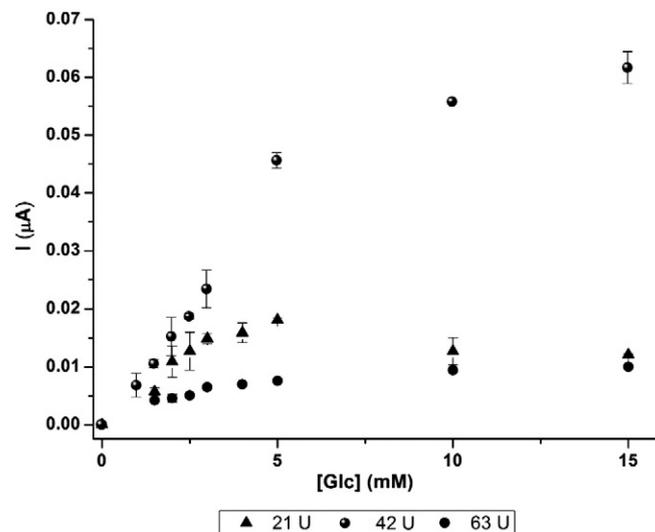
Fig. 4. Effect of enzyme loading on the biosensor response (50 mM, pH 4.0 acetate buffer; 5.0  $\mu\text{L}$  AuNPs; 1.98  $\mu\text{mol}$  FcSH; +0.35 V).
