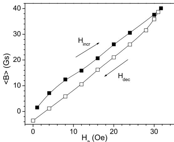
**Figure 3.** Applied field dependence of the average local magnetic induction ( $\langle B \rangle$ ), for increasing and decreasing applied fields, as inferred from SHPM scans.
