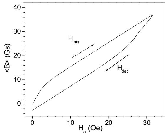
**Figure 4.** Numerical simulation of experimental data shown in figure 3, using equations (1) and (2), for  $H_c = 4$  Oe and  $y = 0.97$  mm.
