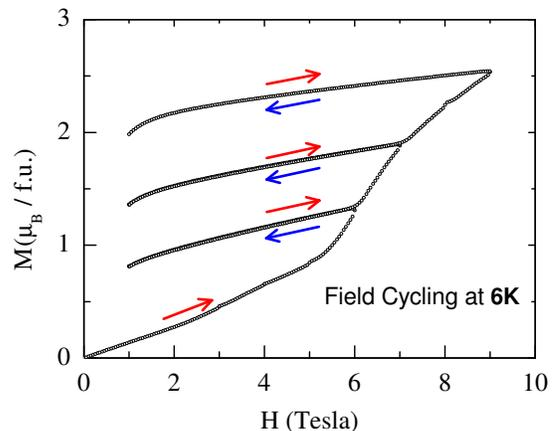
FIG. 4: (color online) Magnetization ( $M$ ) vs. Magnetic field ( $H$ ) at 6 K corresponding to MFM images shown in Figure 2. Irreversible isothermal transformation (devitrification) from AF-I to FM-M state is highlighted.
