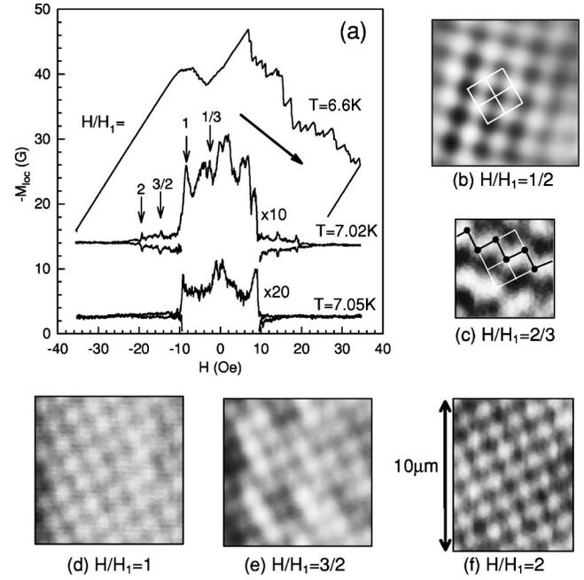
FIG. 2. (a) “Local magnetization” loops (offset for clarity) measured with a Hall probe above the antidot array at three different temperatures. SHPM scans after field-cooling to 5.5 K in (b)  $H=H_1/2$  (white lines indicate the location of four unit cells of the antidot lattice), (c)  $H=2H_1/3$  (black lines and symbols indicate the positions of one chain of flux lines, white lines outline four unit cells of the antidot lattice), (d)  $H=H_1$ , (e)  $H=3H_1/2$ , and (f)  $H=2H_1$ .
