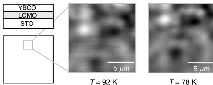
**Figure 1.** Sketch of the sample (left) and maps of the magnetic induction above the sample at temperatures above and below the superconducting transition. The grayscale spans  $-2.5$  to  $2.5$  G. After accounting for a small shift of the measurement area as the temperature is reduced, very similar magnetic structures are observed in both images.
