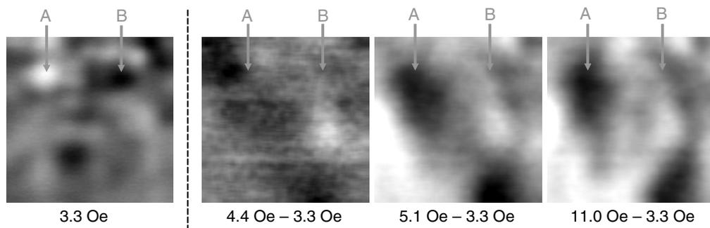
**Figure 4.** Difference images generated from the data of figure 3. The image at  $H_{\text{ex}} = 3.3$  Oe has been subtracted from the images at higher fields to highlight the changes due to flux penetration into the superconductor. All images are optimized to maximum contrast.
