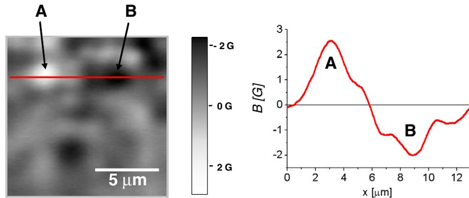
**Figure 2.** Left: SHPM image after zero-field cooling to a temperature of  $T = 78$  K, the scale bar indicates the local magnetic induction. A and B mark two regions with out-of-plane oriented magnetic fields. Right: Line-scan of the magnetic induction across regions A and B along the solid horizontal line on the image.
