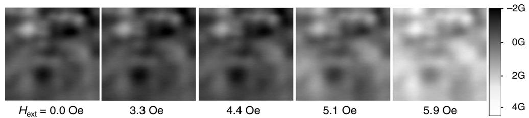
**Figure 3.** SHPM images of the area shown in figure 2 in increasing positive external magnetic fields. The penetration of magnetic flux into the sample is visible as brightening of the images starting from  $H_{\text{ext}} = 4.4$  Oe onwards. Owing to our measurement geometry all magnetic flux lines have to penetrate from the top edge of the image which is closest to the physical edge of the sample.
