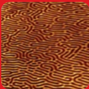
Magnetic domains of garnet single crystal at 300K
