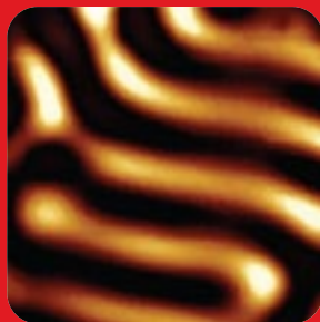
Magnetic domains of garnet single crystal at 1.9K
