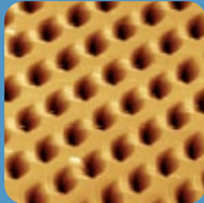
STM Image of 2 μm pitch Calibration Grating
